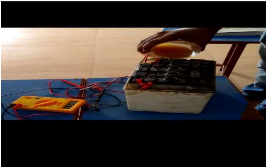
Figure 4: Experiment with cow urine blended with H 2 SO 4 to check the voltage produced
